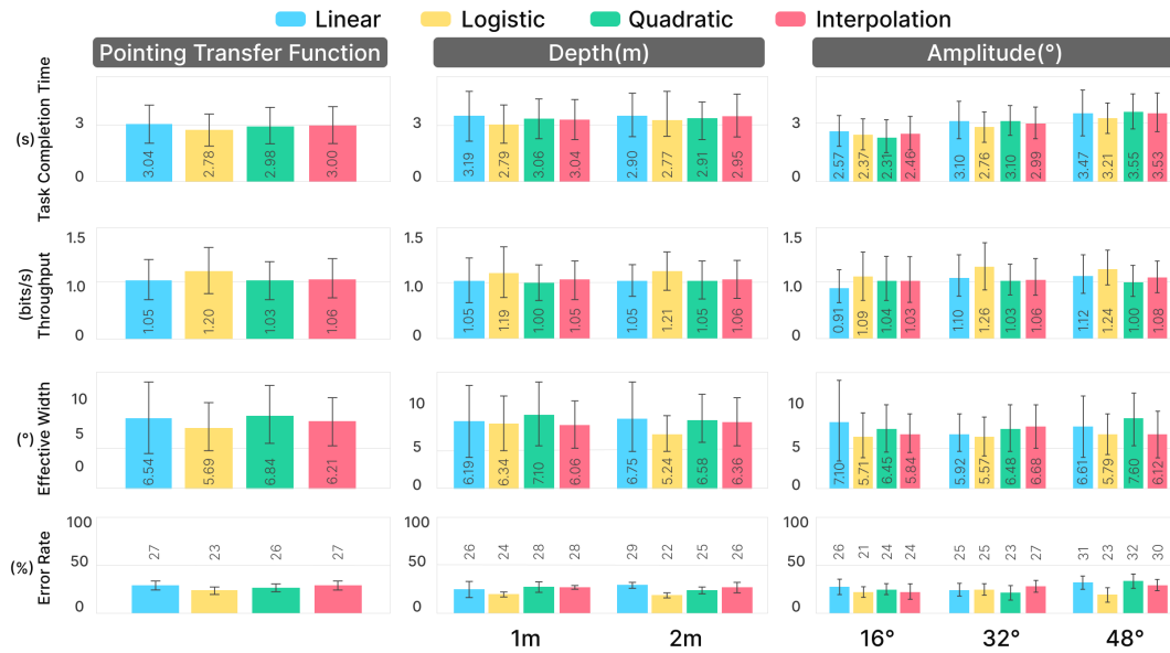
Figure 6: The results of Fitts' law study. The mean values for task completion time, throughput, effective width, and error rate were computed for each transfer function, depth per transfer function, and amplitude per transfer function.
